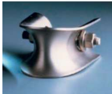
Reverse U-bend (RUB) specimen for tubes
