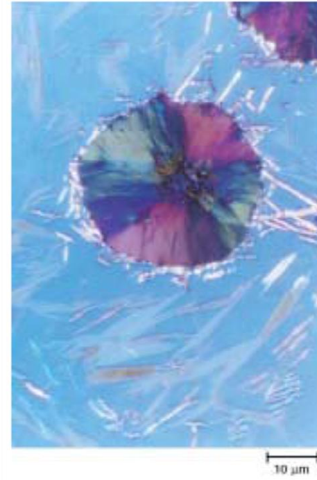
Fig. 54 Same as in Fig. 33 but microstructure was examined in crossed polarized light. Acicular ferrite is shining brightly; plate martensite is slightly gray-blue. 1000×
