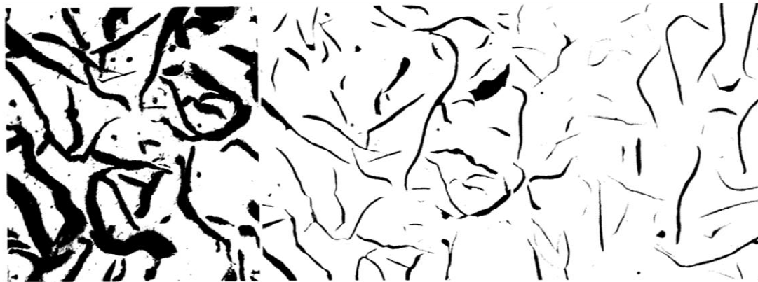
Fig. 49, 50, 51 Comparison of polishing methods for retention of graphite in gray iron. Fig. 49: results of polishing on 10- to 20- \mu\text{m} \text{Al}_2\text{O}_3 on long-nap billiard cloth. Fig. 50: results of polishing on 1- \mu\text{m} diamond on a synthetic suede short-nap cloth. Fig. 51: results of polishing on 1- \mu\text{m} diamond on cotton drill. All specimens were abraded on a fixed-abrasive lap before polishing. As-polished. 250 \times
