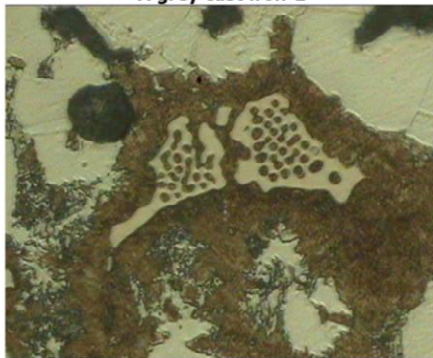
A nodular cast iron- Pearlite- ferrite- ledeburite
