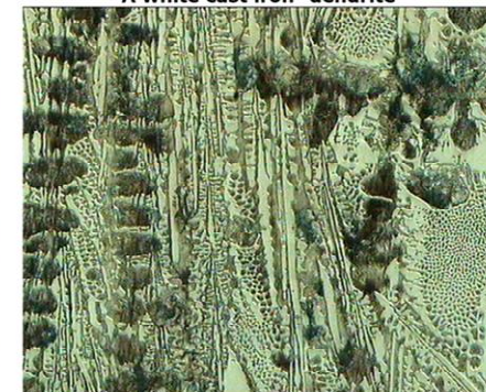
A white cast iron- ledeburite
