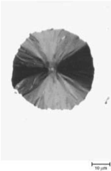
Fig. 51 Graphite nodule examined in bright-field illumination. As-polished. 1000×
