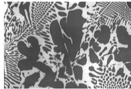
BSE image from flat surface of an Al ( Z=13 ) and Cu ( Z=29 ) alloy
