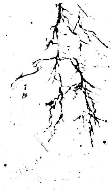
Figure 3-53 Cross section of stress-corrosion crack in stainless steel (500 \times ).
