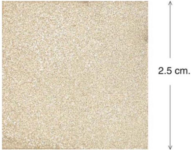
Fig. 2.13 The uniform corrosion of zinc after immersion in hydrochloric acid
