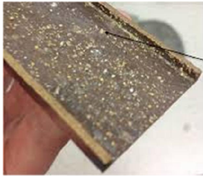
Copper Deposits on the surface of the brass
