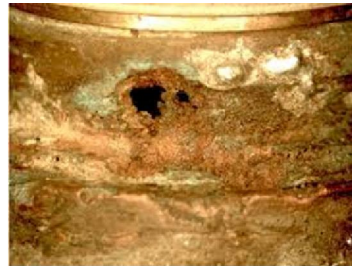
Copper Deposits on the surface of the brass
