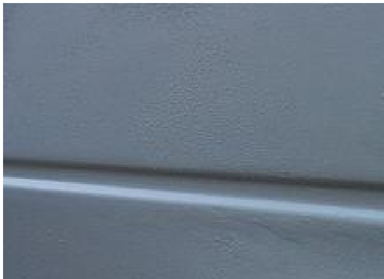
Primer as a step in the coating process of a car body
