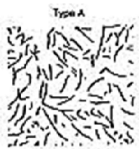
Type A Uniform distribution, random orientation
