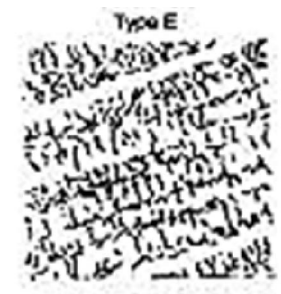
Type E Interdiffusive segregation, preferred orientation
