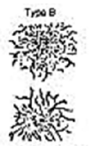
Type B Flake grouping, random orientation
