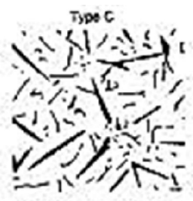
Type C Superimposed flake size, random orientation
