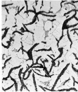
Gray iron \alpha Fe and graphite flakes
