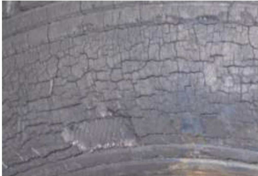
Figure 2. Photo showing ozone cracking of a bias ply tire.
