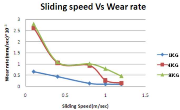
Wear rate of Ti-6Al-4V under ambient condition at 1kg,4kg and 8kg
